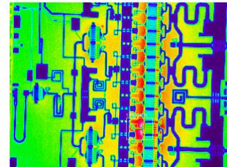
Unpowered devices are placed on the thermal stage and controlled to a stable temperature. The Emissivity Table software is then used to create an emissivity map of the device, allowing accurate temperatures can be obtained at any point on a device.
