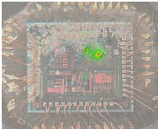
Test sensitivity is directly dependent upon lock-in test time. As a test continues to run, lower and lower power dissipation levels can be detected. There is no limitation on how long a Sentris lock-in test can be performed. Consequently, finding an extremely small heat signature is only a matter of time.
