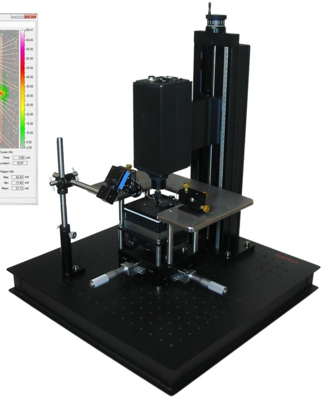
Using a non-destructive testing (NDT) process called lock-in thermography, failures can be isolated on both bare (front or backside) and packaged devices and no surface coating is required. Sentris can also locate low-power fail sites on SMD components, such as capacitor leakage. The x, y position of defect sites can be located, as well as defect depth. Depth analysis can be very helpful when isolating faults in stacked die packages.
