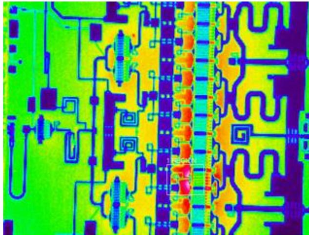
Figure 3 – Thermal image of unpackaged device
