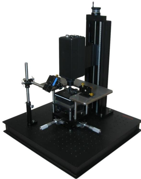
**Figure 1 – Sentris thermal emission microscope**
